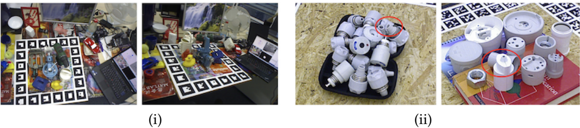
(b) Challenges of cluttered background and occlusions: (i) cluttered environment in Linemod [46], (ii) heavy occlusions for testing objects highlighted in red circle in T-LESS [54].
