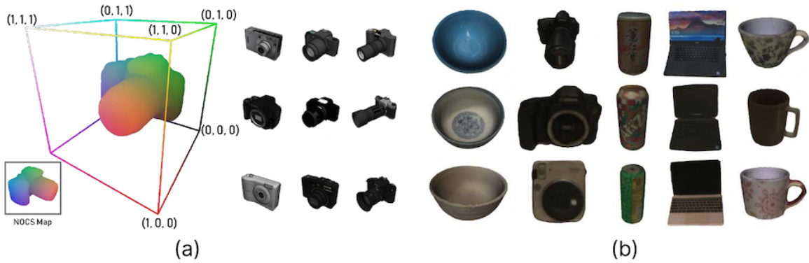
Figure 2.17: Category-level pose estimation with normalized object coordinates in [143] . The normalized object coordinate space, which is contained within a unit cube, displays a 3D space for each category. Within this shared space, all instances of a given category, such as cameras, are aligned in terms of orientation, while their sizes are normalized to fit within the unit cube. This allows for direct prediction of 2D-3D correspondences for novel objects that belong to a known category. As shown in (b), example categories include bowls, cameras, cans, laptops, and mugs. Image taken from [70]. See Section 2.4.1.
